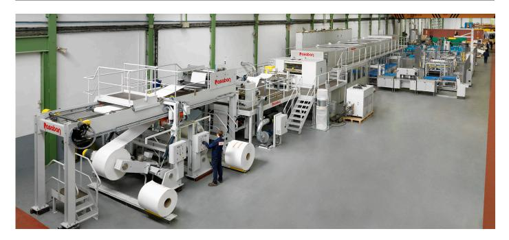
Double Rotary sheeter designed for security cut-to-register paper with the highest precision. The double rotary cutting system provides the best cutting quality in the market.
